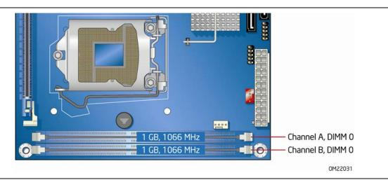
Figure 14. Dual Channel Memory Configuration Example
